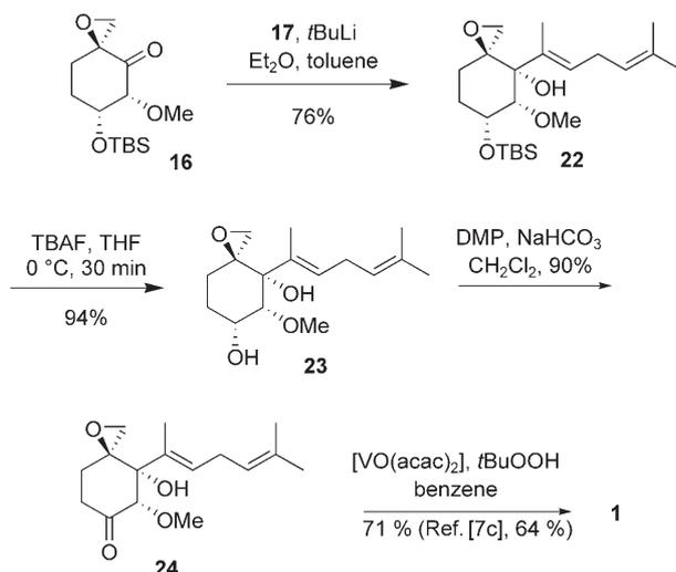
**Scheme 8.** Completion of total synthesis. TBAF = tetra-*n*-butylammonium fluoride, [VO(acac)<sub>2</sub>] = vanadyl acetylacetonate.
