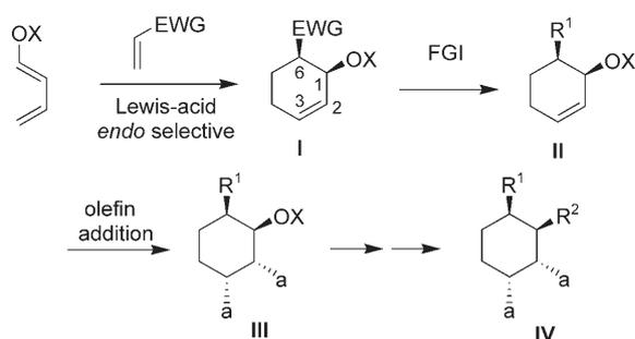
**Scheme 1.** Strategy to reach highly functionalized cyclohexane derivatives. EWG = electron-withdrawing group, FGI = functional-group interconversion, X = SiR<sub>3</sub>, acyl, alkyl.
