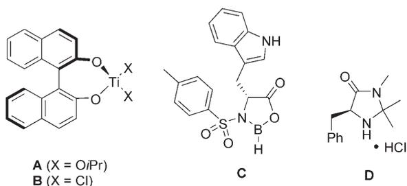
**Scheme 4.** Chiral catalysts tested for the enantioselective Diels–Alder reaction.
