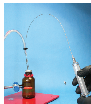
Fig. 8 Filling syringe using nitrogen pressure
