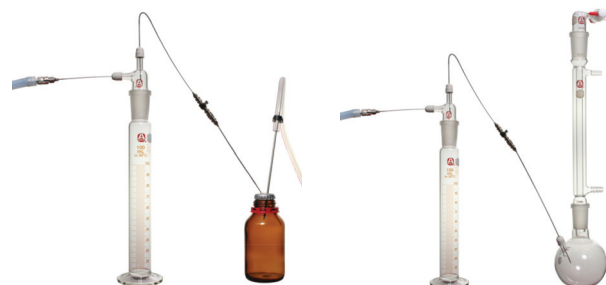
Fig. 12 Double-tipped needle transfer to graduated cylinder
