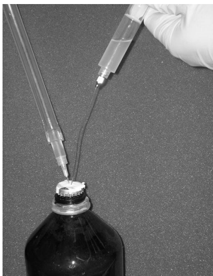
Fig. 1 Drawing reagent into syringe from reagent container, with inert gas line inserted
