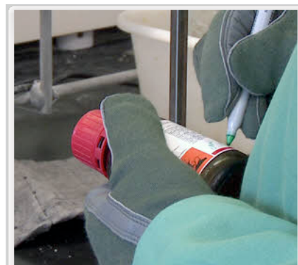
Reagent bottles must be dated when first opened so you will know when to dispose of them
