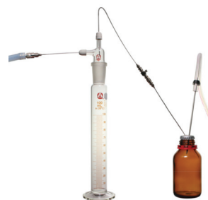
Fig. 12 Double-tipped needle transfer to graduated cylinder
