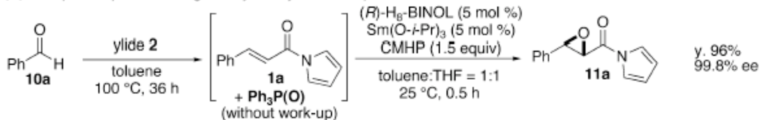
(A) One-pot Sequential Wittig-Catalytic Asymmetric Epoxidation Process
